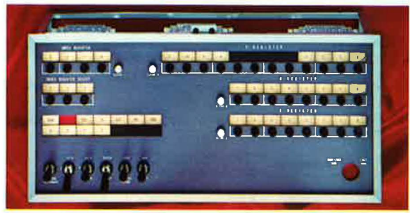
DATA-PANEL and switches are combined in this display-control assembly built for Control Data Corporation.
